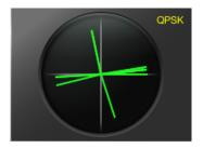
Tuned Correctly (QPSK Mode)
