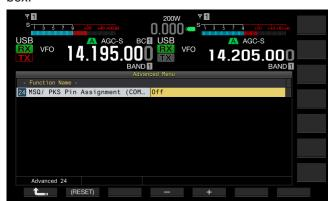
4 Press [-] (F4) or [+] (F5) to select "On" or "Off" to determine the pin behavior.
