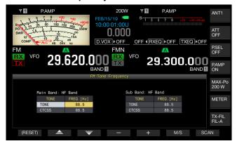
2 Press [M/S] (F6) to select either main band or subband.
