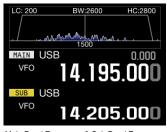
Main Band Frequency & Sub Band Frequency Audio Scope & Bandscope Display
