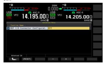
4 Press [-] (F4) or [+] (F5) to select the behavior of the REF I/O (10 MHz) connector from "Off", "Output", or "Input".
